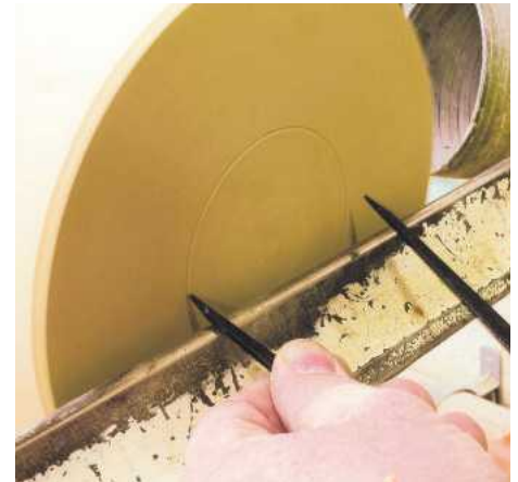
▲ Pic.3 Mark the size of the chuck spigot on the bottom. The larger than usual flat on the bowl will make it more stable
